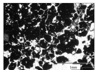
Figure 5 - Photomicrograph showing the fissuration of the porphyroenaulic related distribution (arrows).
