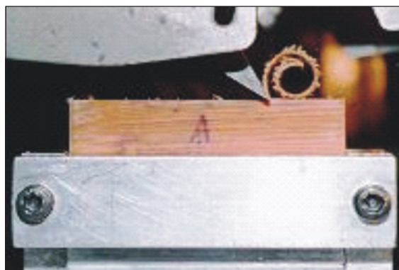
Figure 8 - Type II chip obtained in the 90-0 orthogonal cutting assay. Species: Eucalyptus grandis , cutting thicknesses: 0.38 mm, and angle of attack: \alpha = 30^\circ . (Néri, 1998)
