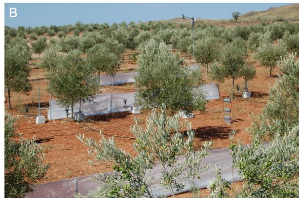
Figure 1 – Olive field in Tabernas (Spain) with an anti-erosion windbreak. Anemometers around the windbreak (A); Situation of the three windbreaks used during the experimental tests (B).
