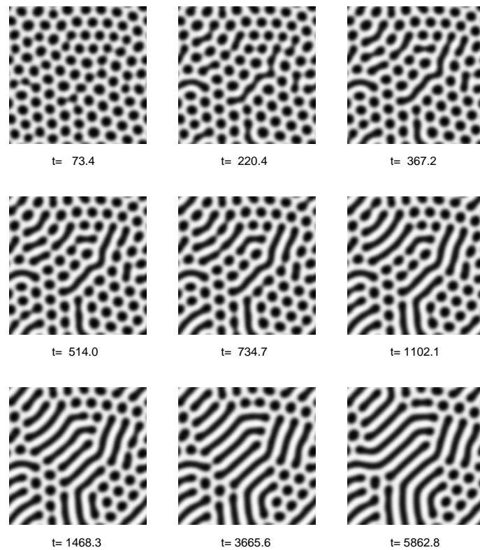
Figure 5. Transformation of the hexagonal structure to the stripe structure at the decrease of the mean concentration. \frac{Bm}{Bm_c} = 0.78 , \frac{h}{l} = 5 , \phi_0 = 0.05 . Initial pattern - the hexagonal structure formed at \frac{Bm}{Bm_c} = 0.78 , \frac{h}{l} = 5 and \phi_0 = 0.2 .
