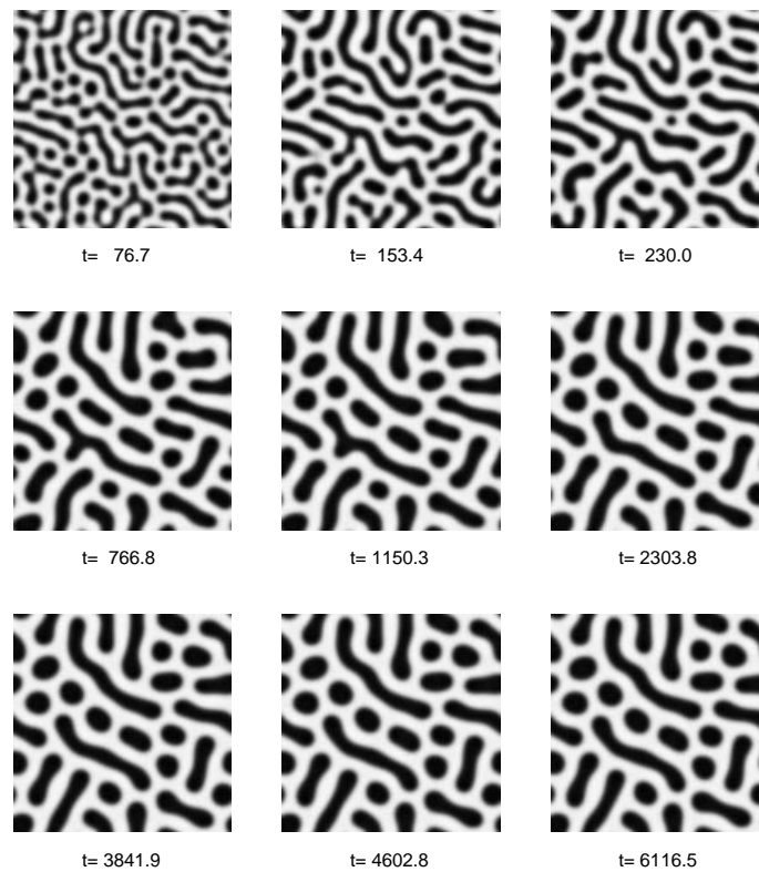
Figure 6. Mixed intermediate state of the magnetic colloid ( \frac{Bm}{Bm_c} = 0.3 , \frac{h}{l} = 10 , \phi_0 = 0.075 ).
