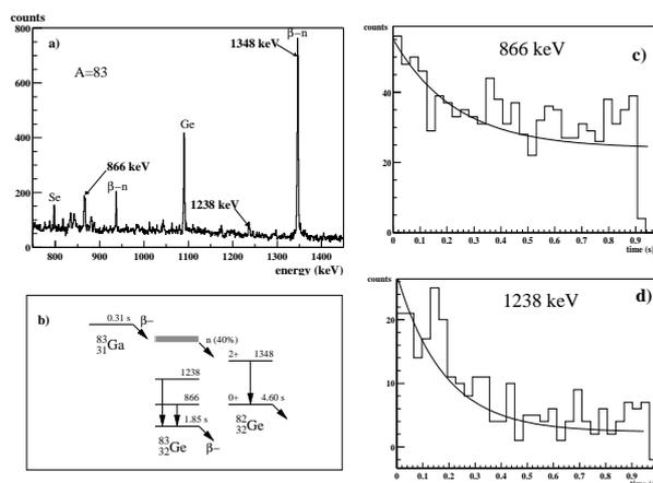
Figure 2. a) Part of the  $\gamma$ -ray spectrum measured at mass 83 in  $\beta$  coincidence. b) Schematic representation of some of the observed transitions fed in the  $^{83}\text{Ga}$  decay. c) Time spectrum and fitted decay curve for the line at 866 keV, the deduced period is  $250 \pm 161$  ms. d) Time spectrum and fitted decay curve for the line at 1238 keV, the deduced period is  $260 \pm 140$  ms.
