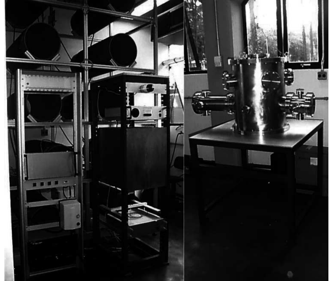
Figure 9. General view of the Blumlein pulser (left) and the plasma chamber (right).
