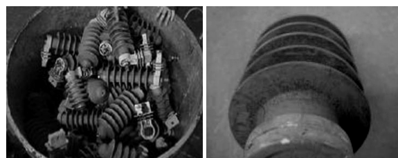
Figure 2. SR surge arresters and insulators with problems taken from the field.
