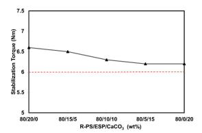
**Figure 2.** Stabilization torque of ESP/CaCO<sub>3</sub> hybrid filled R-PS composites (Red dash-line is for stabilization torque of neat R-PS).
