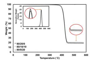
Figure 9. TG and DTG curves of ESP/CaCO<sub>3</sub> hybrid filled R-PS composites.
