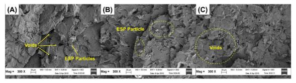
Figure 8. Impact fractured surfaces of ESP/CaCO<sub>3</sub> hybrid filled R-PS composites at 300× magnification. 80/20/0 wt% (A), 82/10/10 wt% (B) and 80/0/20 wt% of R-PS/ESP/CaCO<sub>3</sub> respectively.
