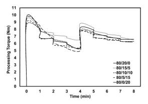
**Figure 1.** Processing torque as a function of mixing time of ESP/CaCO<sub>3</sub> hybrid filled R-PS composites.
