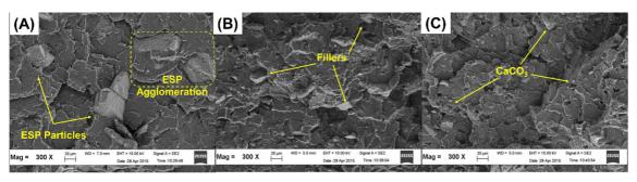
Figure 7. Tensile fractured surfaces of ESP/CaCO $_3$  hybrid filled R-PS composites at 300× magnification. 80/20/0 wt% (A), 82/10/10 wt% (B) and 80/0/20 wt% of R-PS/ESP/CaCO $_3$  respectively.
