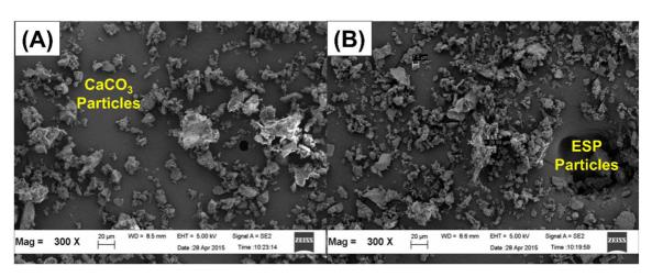
Figure 6. SEM images of raw CaCO<sub>3</sub> and ESP.
