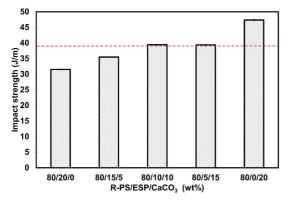
**Figure 5.** Impact strength of ESP/CaCO<sub>3</sub> hybrid filled R-PS (Red dash-line is the impact strength of neat R-PS).
