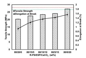
**Figure 3.** Tensile strength and elongation at break of ESP/CaCO<sub>3</sub> hybrid filled R-PS composites (Red and green dash-lines are for the tensile strength and elongation at break of neat R-PS).
