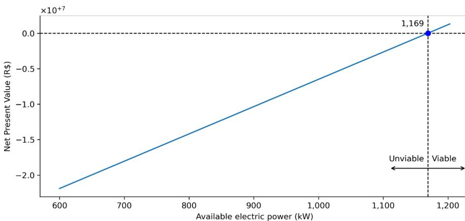
**Figure 5.** Sensitivity analysis: NPV as a function of electric power variations.
