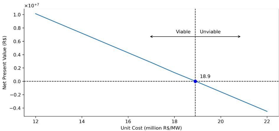
**Figure 7.** Sensitivity analysis: NPV as a function of unit cost variations.
