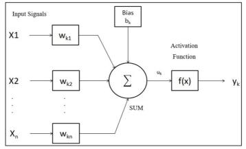
Figure 1. Structure of an artificial neuron.
