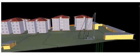
Figure 12. Navisworks software image showing the pile driver installation for elevated water reservoir foundation.
