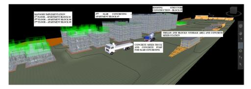
Figure 10. Navisworks software image showing the construction site layout at the critical path main tasks stage.
