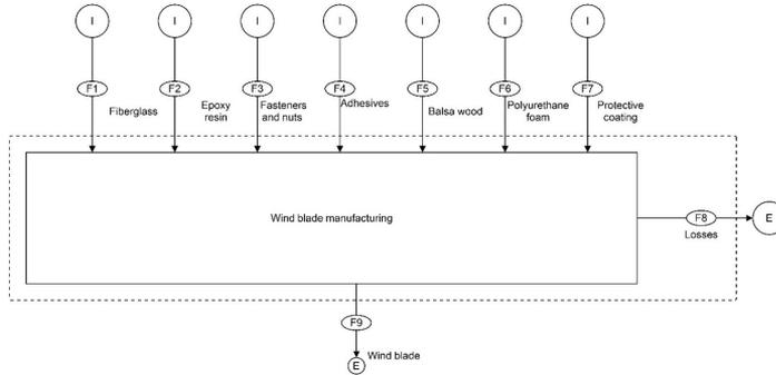
**Figure 1.** Product system: manufacture of wind turbine blades. The flows are classified as import (I) or export (E).
