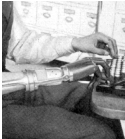
Fig. 3 – A prosthesis built at the Institute which improved the ability of a patient with a hand amputation to typewrite.
