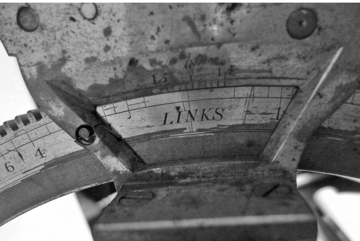
Figure 4: Detail of the nonium (Photo by I. Malaquias)
