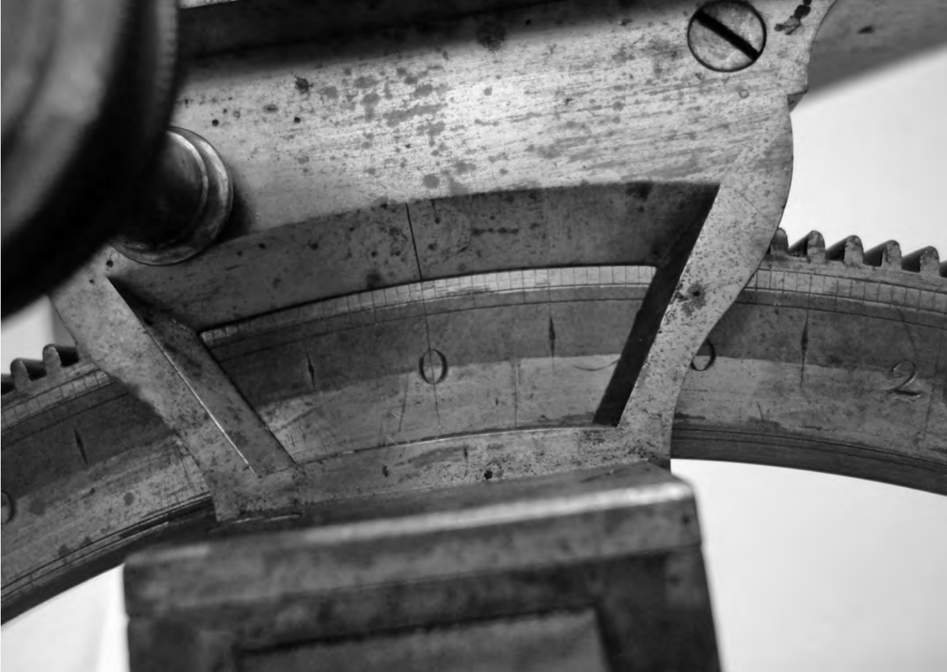
Figure 5: Detail of the vertical nonium opposite side (Photo by I. Malaquias)
