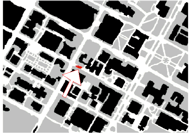
(b) Induced map: free space (white), occupied space (black), and semi-occupied space (gray).
