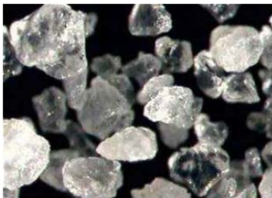
Figure 3: Quartz particles, D_p = 185\mu\text{m} (left) and duroplastic particles, D_p = 240\mu\text{m} (right).
