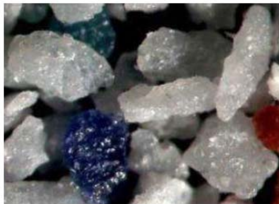
Figure 3: Quartz particles, D_p = 185\mu\text{m} (left) and duroplastic particles, D_p = 240\mu\text{m} (right).
