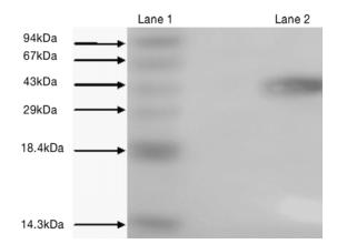
**Figure 1:** Electrophoretogram of protein after various steps of purification on SDSPAGE. Electrophoresis was carried out using a 15 % crosslinked polyacrylamide. Lane 1: standard molecular weight markers; Lane 2: purified enzyme.
