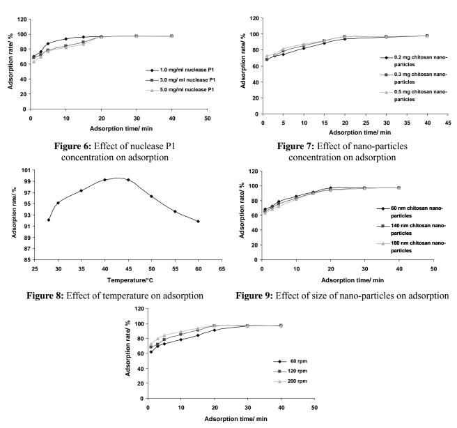
Figure 10: Effect of agitation speed on adsorption
