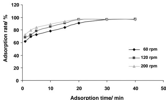
**Figure 10:** Effect of agitation speed on adsorption
