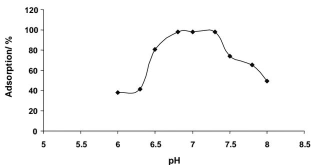
Figure 11: Effect of pH on adsorption
