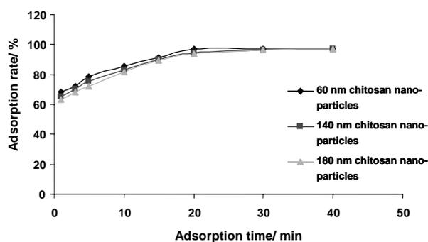
**Figure 9:** Effect of size of nano-particles on adsorption
