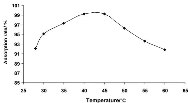
**Figure 8:** Effect of temperature on adsorption
