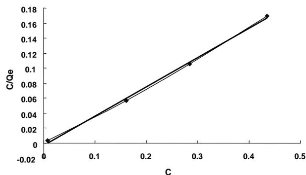
Figure 13: Langmuir adsorption isotherm
