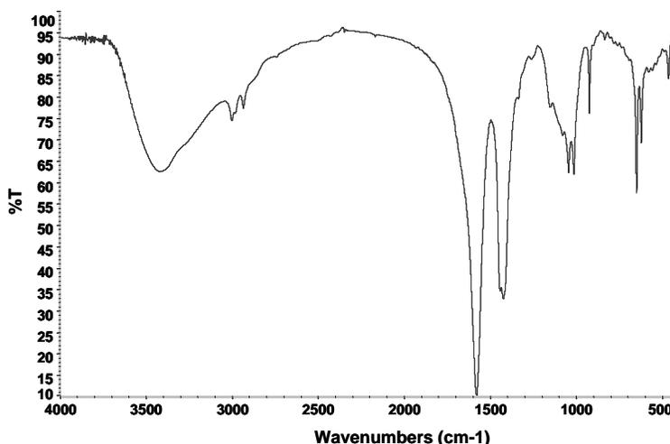
**Figure 5:** Infrared spectra of chitosan nano-particles with adsorbed nuclease P1
