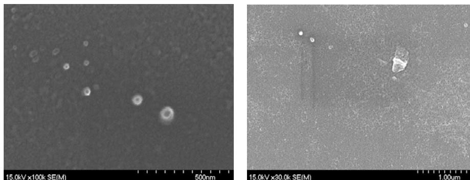
**Figure 2:** SEM of chitosan nano-particles. The size of chitosan nano-particles (60 nm) can be measured by the ruler in Figure 2.
