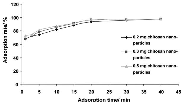
**Figure 7:** Effect of nano-particles concentration on adsorption
