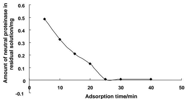
Figure 12: Adsorption isotherm Adsorption temperature:  $30^\circ\text{C}$ ; Agitation speed: 120 rpm; Bulk concentration: 3.0 mg/ml
