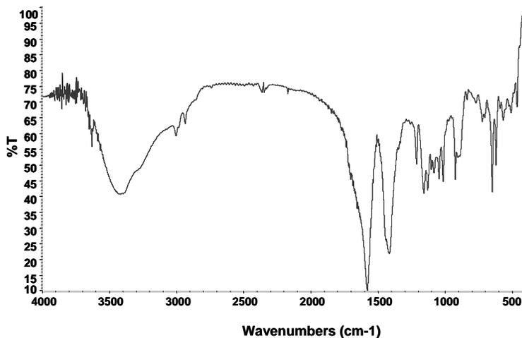
Figure 4: Infrared spectra of chitosan nano-particles
