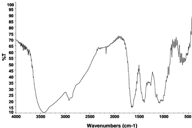
Figure 3: Infrared spectra of chitosan
