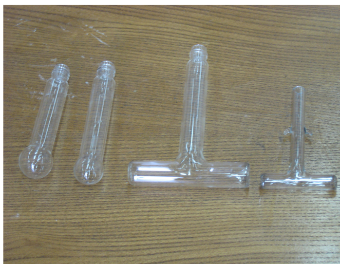
Figure 4: Quartz sample in cylindrical and spherical coordinates for the measurement of volumetric heat generation power due to the infrared radiation
