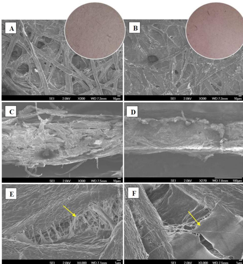
**Figure 1.** FEG-SEM micrographs of papers reinforced with cellulose nanofibrils showing paper surfaces rough (A) and smooth (B) with respective samples, paper thickness (C, D), formation of nanofilm within the paper (E, F). Arrows pointing to zones of nanofilm formation.
