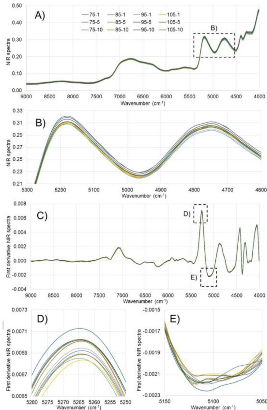
**Figure 2.** Mean raw (untreated, A) and first derivative (C) NIR spectra for each nanofibril content (1, 5 and 10%) and grammage (75, 85, 95 and 105 g m<sup>-2</sup>) of Kraft paper handsheets reinforced with CNF and detailed spectra ranges (B, D and E).
