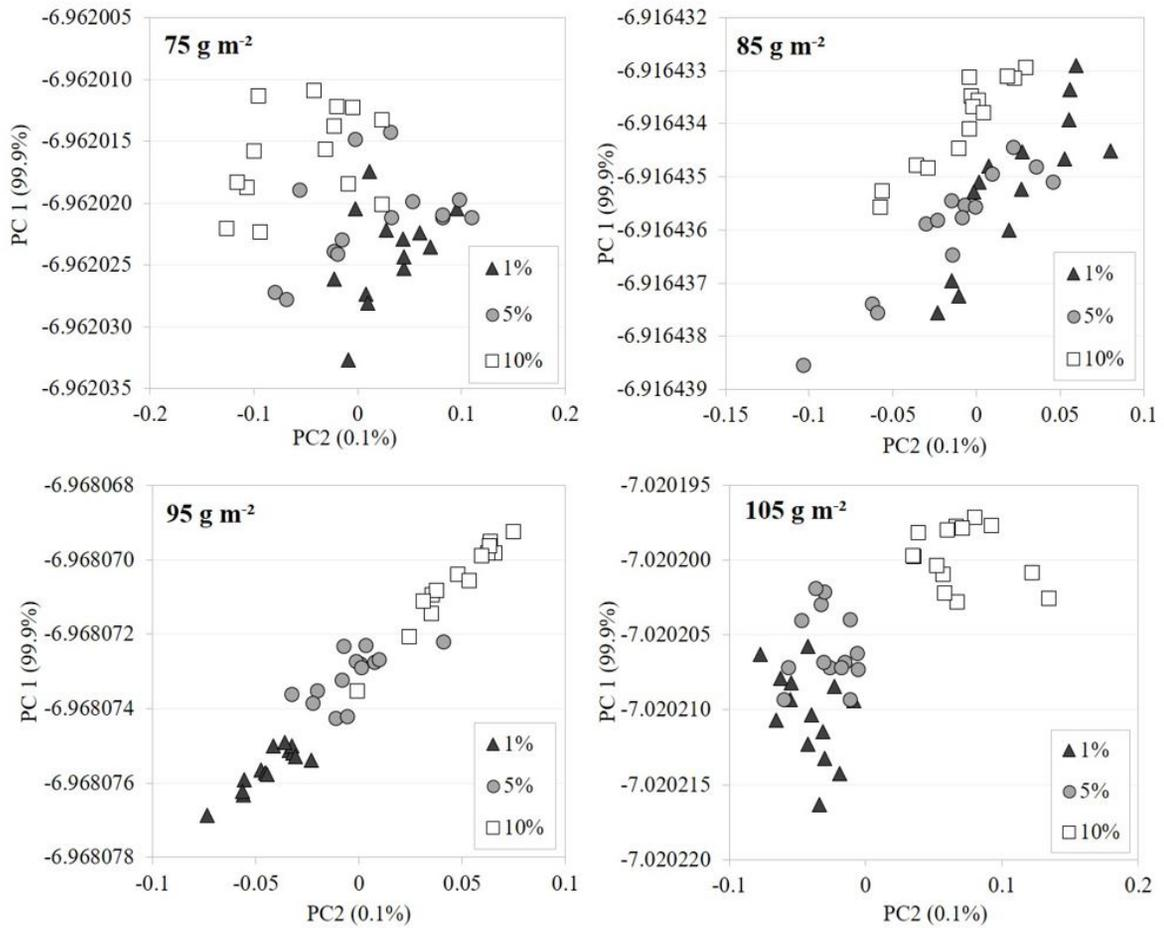
**Figure 4.** Scores of PCAs applied to NIR spectra after Multiplicative Scatter Correction recorded from Kraft paper handsheets reinforced with CNF with nominal grammage of 75, 85, 95 and 105 g. m<sup>-2</sup>.
