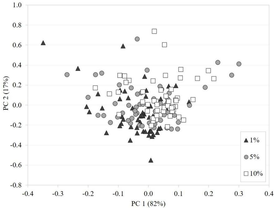
**Figure 3.** Scores of a PCA applied to untreated NIR spectra recorded from Kraft paper handsheets reinforced with CNF.
