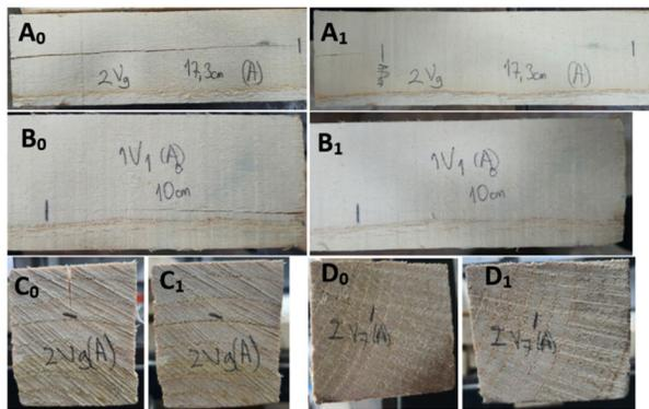
**Figure 11:** Decreasing dimensions (A, C) and closing (B, D) in checks (0: Before, 1: After).
