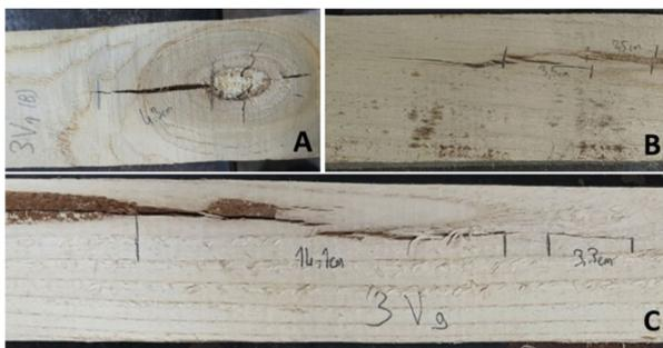
**Figure 12:** Check development on the knot (A) and pith (B & C).
