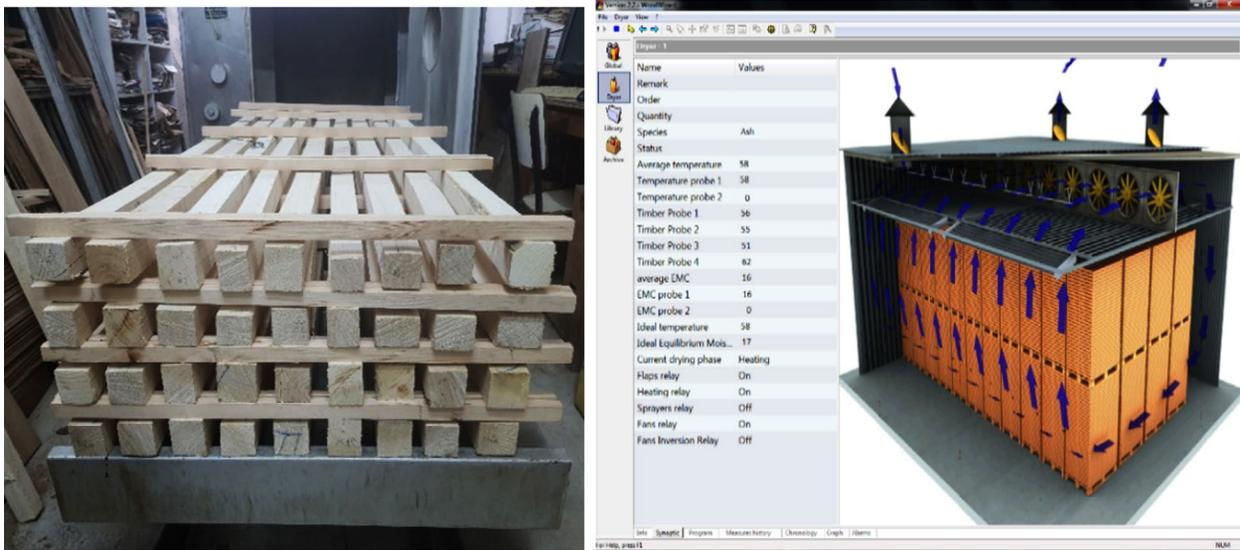
**Figure 3:** Stacking (Left) and a sample screen of drying automation software (Right).
