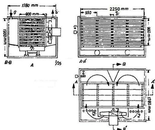
Figure 2: Drying Kiln (Drawing: Ünsal, 1994).
