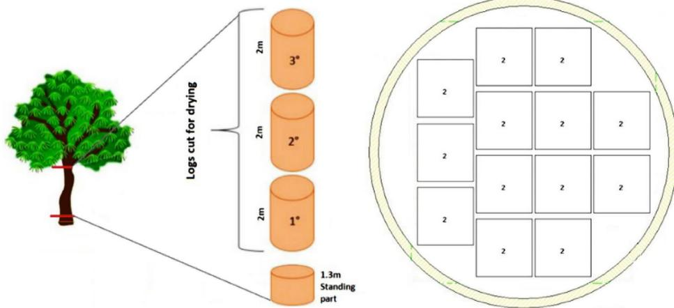
Figure 1: (Left) Log cutting, (Right) Lumber cutting diagram.
