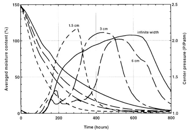
**Figure 4:** Overall drying curve and internal pressure for different widths (Perré and Turne, 1999).
