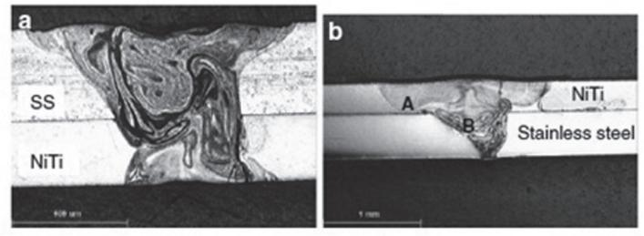
Figure 5. Macrographs of dissimilar welds. a) stainless steel/NiTi weld; b) NiTi/stainless steel
