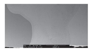
Figure 12. Macrograph of a NiTi/Ti6Al4V weld free of defects
