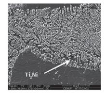
Figure 11. Details of a NiTi/Ti6Al4V weld
