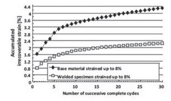
Figure 3. Comparative accumulation of inelastic strain to welded joints and base material strained up to 8%.13]
