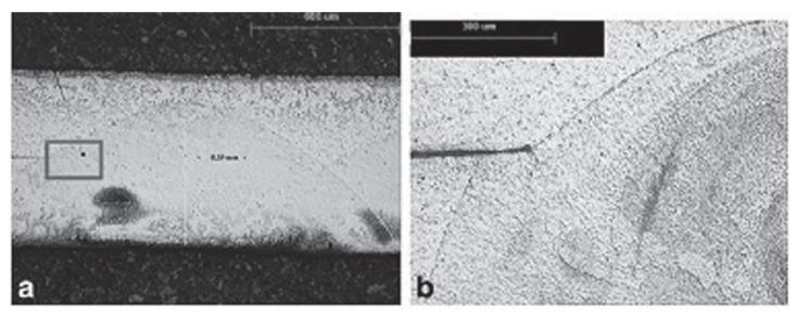
Figure 2. NiTi/NiTi weld of 0.34-mm-thick plates. a) Macrograph / b) weld microstructure. Beam spot diameter = 1 mm, pulse duration =7 ms, energy =9.2 J, power density = 41 830 Wcm<sup>-2</sup>
