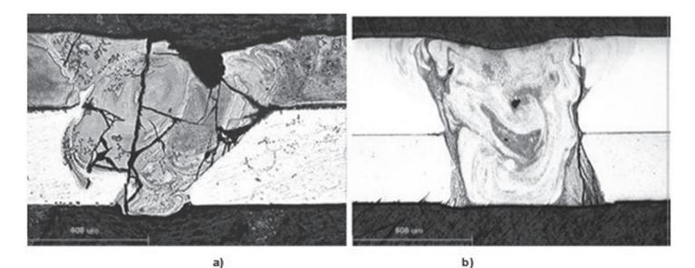
Figure 4. Macrograph of a stainless steel/NiTi weld. Flash lamp, 250 V ; beam spot diameter, 1 mm.
