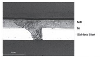
Figure 8. NiTi/Ni (0.05 mm)/stainless steel. Beam spot diameter: 1 mm; flashlamp voltage, 260 V; pulse energy, 30.28 J; pulse duration, 50 ms; intensity, 77.102 W/cm<sup>2</sup>
