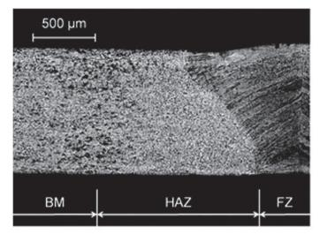
Figure 1. Macrograph of a specimen welded across the rolling direction showing the welded zones (Power: 910 W, welding speed: 25 mm/s)
