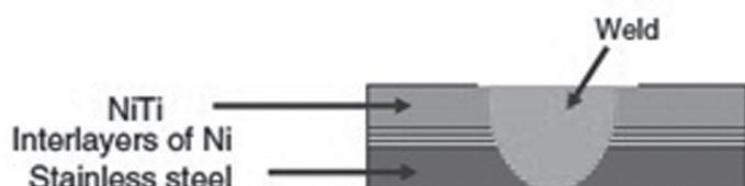
Figure 6. Expected weld shape
