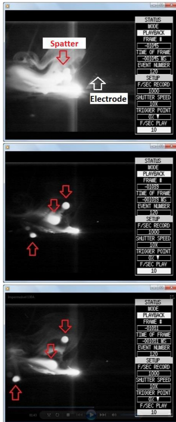
Figure 8. Spatter formation during welding with the polymer-binder electrode at a current of 130 A. Filmed from the side.
