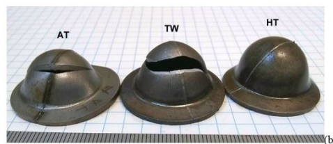
Figure 8. Erichsen cupping test for AT (ambient temperature), TW (tempered weld) and HT (high temperature) coupons: (a) measured stresses versus the depth of the indentation during the test; (b) the final aspect of the coupons at the end of the test. Lower scale in millimeters.
