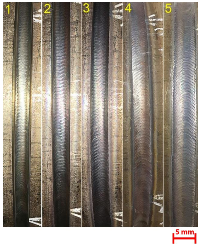
Figure 6. Superficial aspects of filling passes e finishing pass. The numbers from 1 to 5 means the sequence of welding passes.
