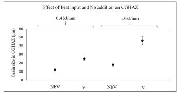
Figure 6. Data distribution for CGHAZ grain size.
