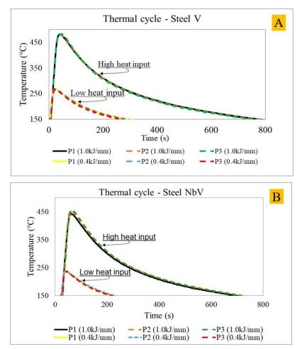
Figure 4. Thermal cycle for welded steels (A) NbV steel (B) V steel.
