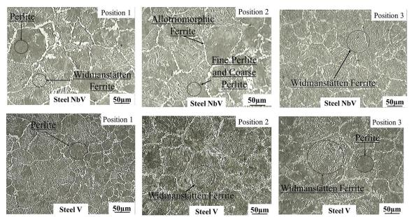
Figure 7. Micrography of CGHAZ at three different positions for high heat input welding.
