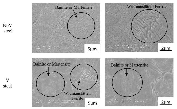
Figure 10. Results for SEM analysis in samples welded at low heat input.
