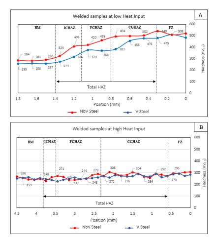
Figure 11. Hardness profiles (A) Welding at low heat input (B) Welding at high heat input.
