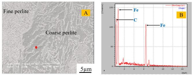
Figure 8. Constituents analyses (A) Micrography of a coarse and fine perlite colony (B) EDS results for a perlite lamella (red point).
