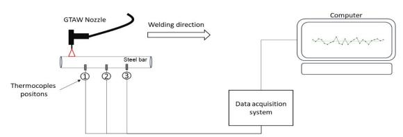
Figure 1. Schematic for GTAW process of steel bar without filler metal and data acquisition system linked to computer. The welding was performed by a travel mechanism automatically.
