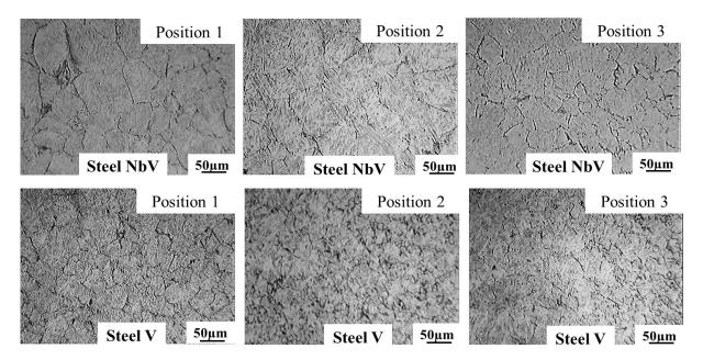
Figure 9. Optical micrography of CGHAZ at three different positions for low heat input welding.
