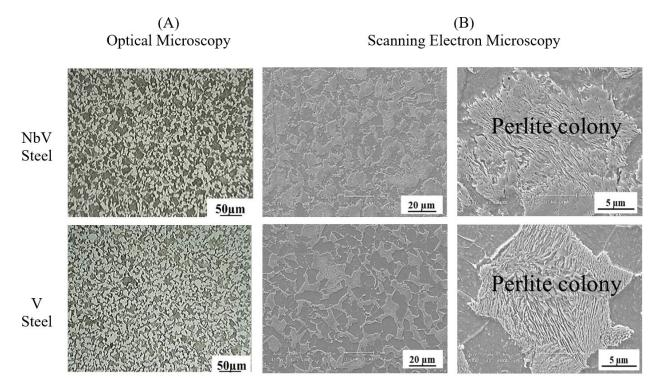
Figure 3. Results for SEM and OM analysis in samples of BM.
