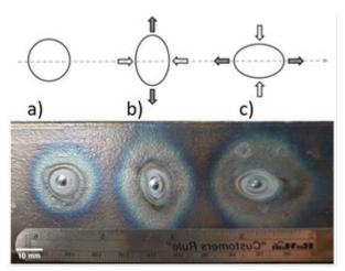
Figure 9. Impressions of the electric arc on sheet.
