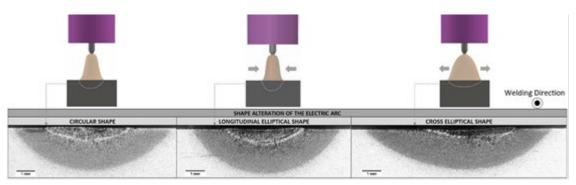
Figure 11. Metallography of the beads on plate and arc shape.
