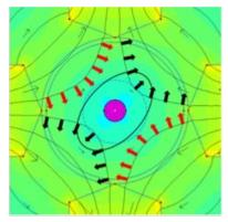
Figure 4. Distribution of forces around the electric arc.
