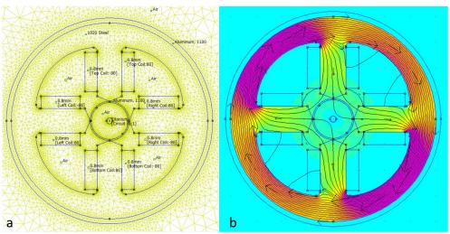
Figure 1. Electromagnetic simulation of the constricting device.
