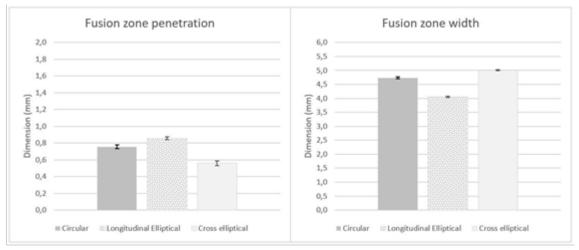
Figure 12. Penetration and width of fusion zone.
