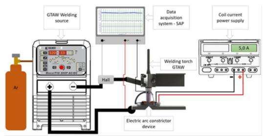
Figure 8. Mounting the constrictor device on the workbench.
