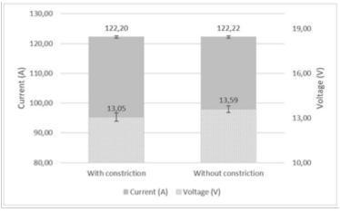
Figure 13. Effect of arc constriction on welding current and arc voltage.
