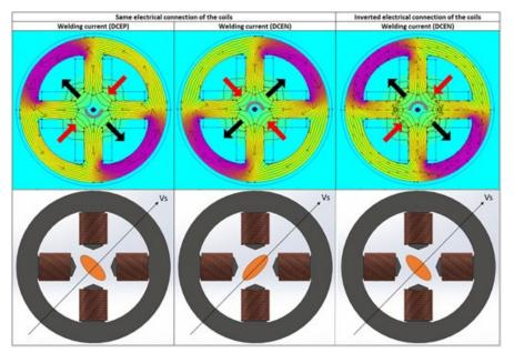
Figure 5. Distribution of traction and compression forces on the electric arc.
