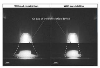
Figure 10. Footage of the electric arc's constriction.
