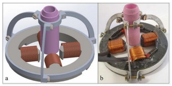
Figure 7. 3D Modeling (a) and manufactured constrictor device (b).
