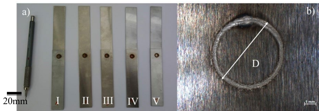
Figure 1 - a) As-welded samples with parameters defined in Table 1; b) Macroscopy of a circular bead produced by a laser beam.
