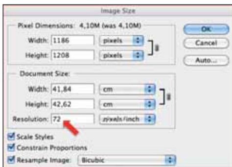
FIGURE 1: Window image size showing the number of pixels and the size of the document
