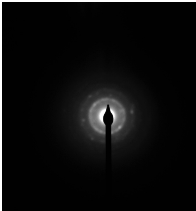
Figure 7: Electron diffraction of the sample's crystalline phase after immersion in SBF.
