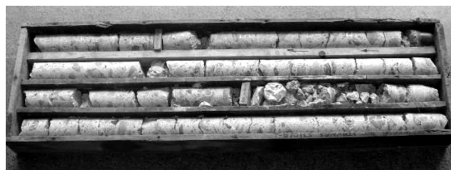
Figure 9: Core samples from 697 to 694 m depth of the dam.
