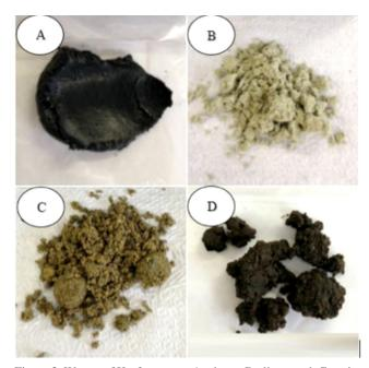
Figure 2: Wastes of Kraft process: A - dregs, B - lime mud, C - grits, and D - pulp mill sludge. [Figura 2: Resíduos do processo Kraft: A - dregs, B - lama de cal, C - grits e D - lama de ETE.]
