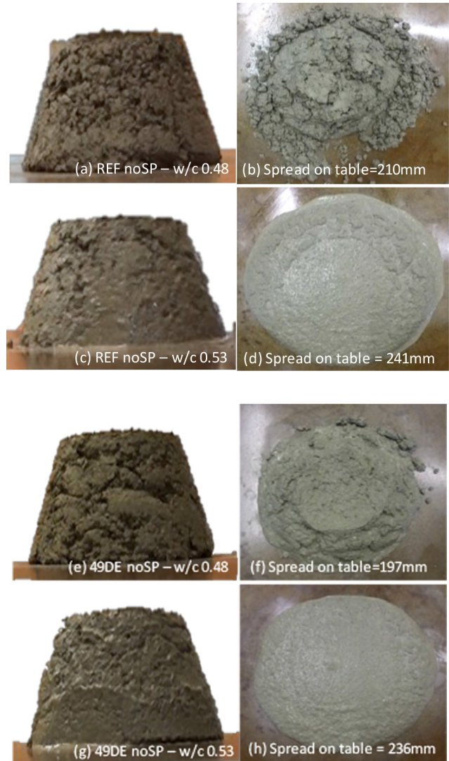
Figure 6: Images before (left) and after (right) the flow table test (dropping the table 30 times) of mortars made with different water/cement (w/c) ratio: a,b) REF mortar with 0.48 w/c; c,d) REF mortar with 0.53 w/c; e,f) 49DE mortar with 0.48 w/c; and g,h) 49DE mortar with 0.53 w/c.
