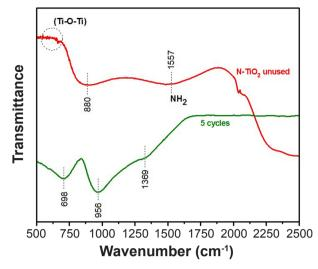
Figure 8: FTIR spectra of N-doped  $\text{TiO}_2$  film grown by MOCVD before and after 5 photocatalytic dye degradation cycles under visible light.
