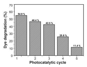
Figure 7: Five recyclability cycles of photocatalytic degradation for methyl orange in the presence of 2.44 at% N-doped TiO<sub>2</sub> film under visible light for 300 min at pH=2. The photocatalytic reactivation of the film surface was performed with ethyl alcohol for 10 min at room temperature and drying in N<sub>2</sub> after each cycle.
