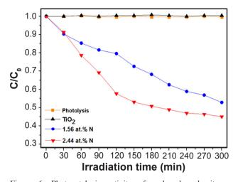
Figure 6: Photocatalysis activity of undoped and nitrogendoped  $\text{TiO}_2$  films grown by MOCVD on the methyl orange dye degradation under visible light irradiation for 300 min.
