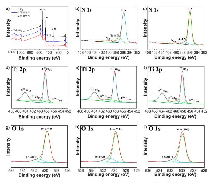
Figure 1: XPS spectra of undoped and N-doped  $\text{TiO}_2$  films grown on borosilicate glass substrates at 400 °C by MOCVD: XPS survey spectra (a) and high-resolution XPS spectra of: N 1s region with fitted curves for 1.56 at% N (b), and 2.44 at% N (c) films; Ti 2p region with fitted curves for undoped (d), 1.56 at% N (e), and 2.44 at% N (f) films; and O 1s region with fitted curves for the undoped (g), 1.56 at% N (h), and 2.44 at% N (i) films.
