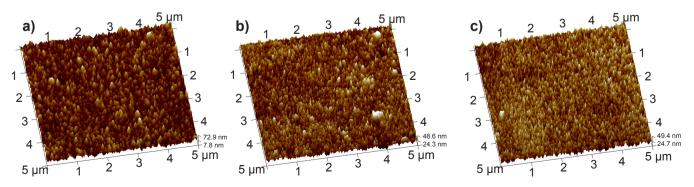
Figure 4: AFM topography images of undoped (a), and 1.56 at% (b), and 2.44 at% (c) N-doped TiO<sub>2</sub> films grown by MOCVD. [Figure 4: Imagens topográficas de AFM dos filmes de TiO<sub>2</sub> não dopado (a) e dopado com 1,56 at% de N (b) e 2,44 at% de N (c) crescidos por MOCVD.]
