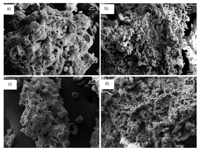
Figure 3: SEM images of the samples before (a,b) and after (c,d) the incorporation of the nanoparticles.
