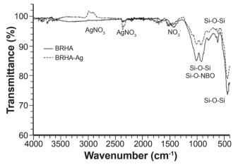
Figure 2: ATR-FTIR spectra for the samples before and after the addition of silver nanoparticles.
