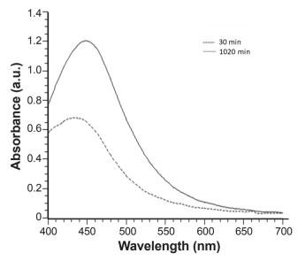
Figure 1: UV-vis spectra from silver nanoparticles after 30 and 1020 min of formation.
