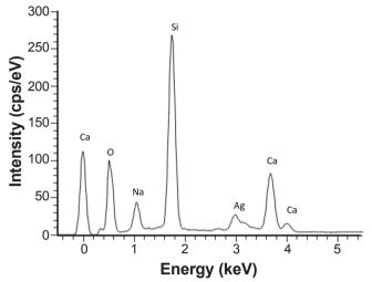
Figure 4: EDS spectrum for the sample after the incorporation of the silver nanoparticles.
