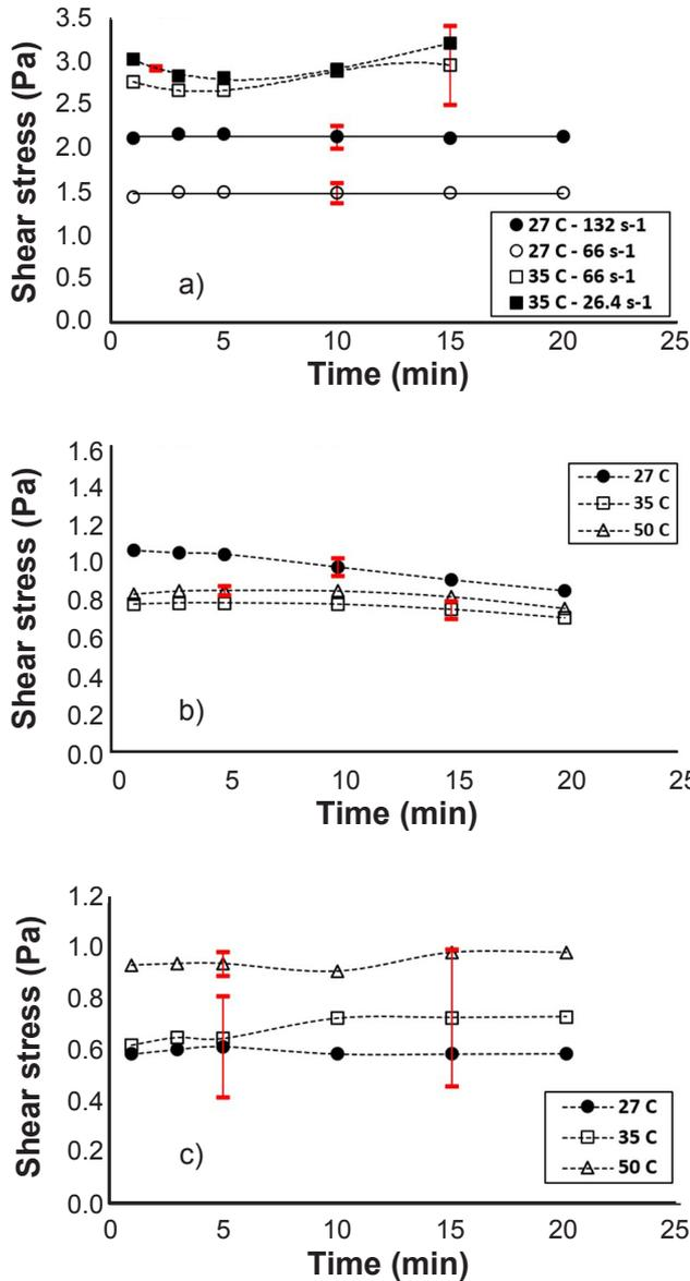
Figure 6: Shear stress as a function of time at constant shear rate and temperature: a) HM-B32 pulp; b) HM-B32-1 pulp at  $\dot{\gamma}=66 \text{ s}^{-1}$ ; and c) HM-B32-3 pulp at  $\dot{\gamma}=66 \text{ s}^{-1}$  (lines link data without any statistical treatment).
