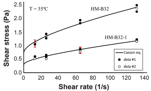
Figure 7: Typical shear stress as a function of shear rate curves at a constant temperature of 35 °C, for HM-B32 and HM-B32-1 pulps (data #1:  $\tau$  vs.  $\dot{\gamma}$  average values for the two first cycles; data #2:  $\tau$  vs.  $\dot{\gamma}$  average values for the last cycle; full line curves: best fitting of Casson model to data).
