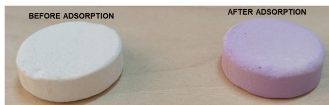
Figure 7: Representative photograph of  $\text{Nb}_2\text{O}_5$  pellets before and after adsorption of methylene blue.
