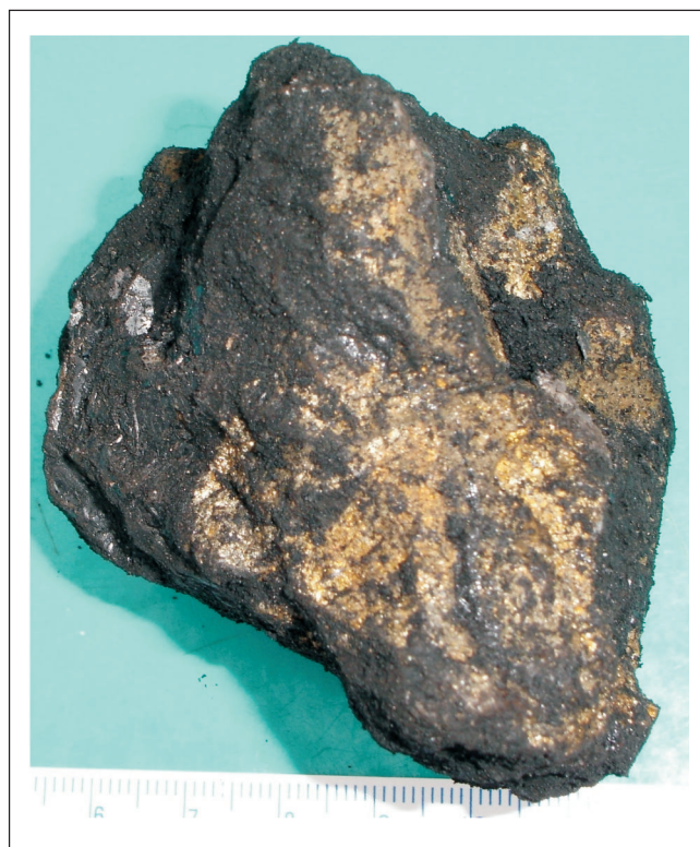
Figure 1 - Coal fragment with pyrite (yellow). The scale's smaller traces indicate millimeters.
