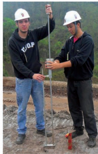
Figure 1 DCP scheme and its operation.
