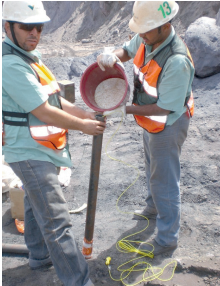
Figure 2 Loading the mix in the steel pipe Schedule 80.
