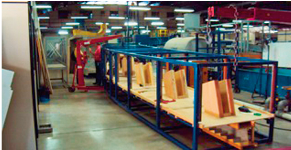
Figure 4 Hillside culvert surrounded by metal framework that will support the structure for the reduced model
