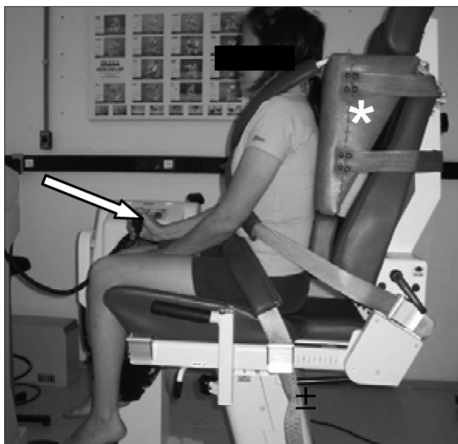
Figure 1. Positioning of the volunteer in the seat of the dynamometer: device (arrow) that was used to start or stop the passive evaluation, and accessory (*) to keep the hip joint at 90° of flexion, respectively.
