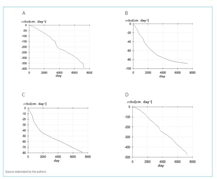
Figure 5 - Graphical representation of the accumulated bottom flux for the four coverage layers of the landfill: (A) vegetation cover by grass; (B) vegetation cover by brachiaria; (C) capillary barrier coverage; (D) compact soil coverage.
