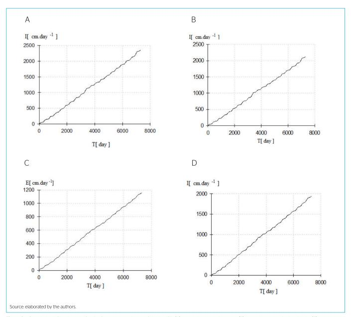
Figure 3 - Cumulative infiltration rate for the four coverage layers of the landfill: (A) vegetation cover by grass; (B) vegetation cover by brachiaria; (C) compact soil coverage; (D) capillary barrier coverage.
