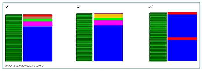
Figure 2 - Profiles 1D: (A) vegetation cover (grass or brachiaria); (B) capillary barrier; (C) compact soil.
