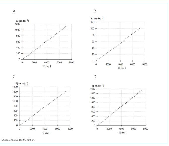
Figure 4 - Cumulative evaporation rate for the four coverage layers of the landfill: (A) vegetation cover by grass; (B) vegetation cover by brachiaria; (C) capillary barrier
