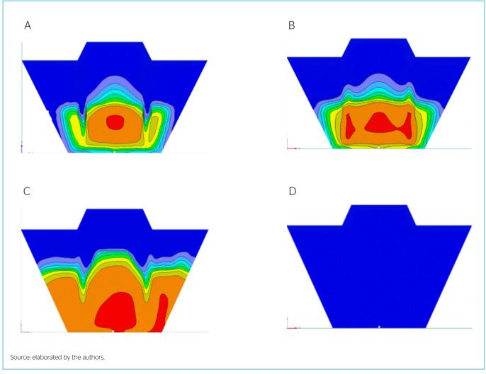
Figure 7 - Contaminant behavior over the time frame of 20 years by means of instant photographs for the four coverage layers of the landfill: (A) vegetation cover by grass; (B) vegetation cover by brachiaria; (C) capillary barrier coverage; (D) compact soil coverage.
