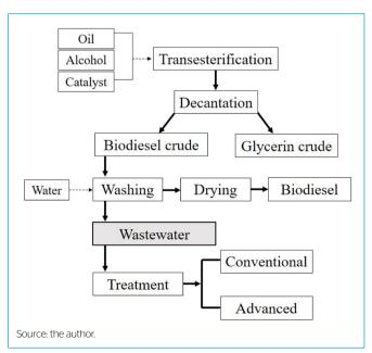
Figure 1 - Biodiesel production stages up to wastewater generation.
