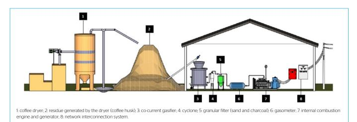
Figure 3 - Electricity production from gasification process (LUZ, 2013).
