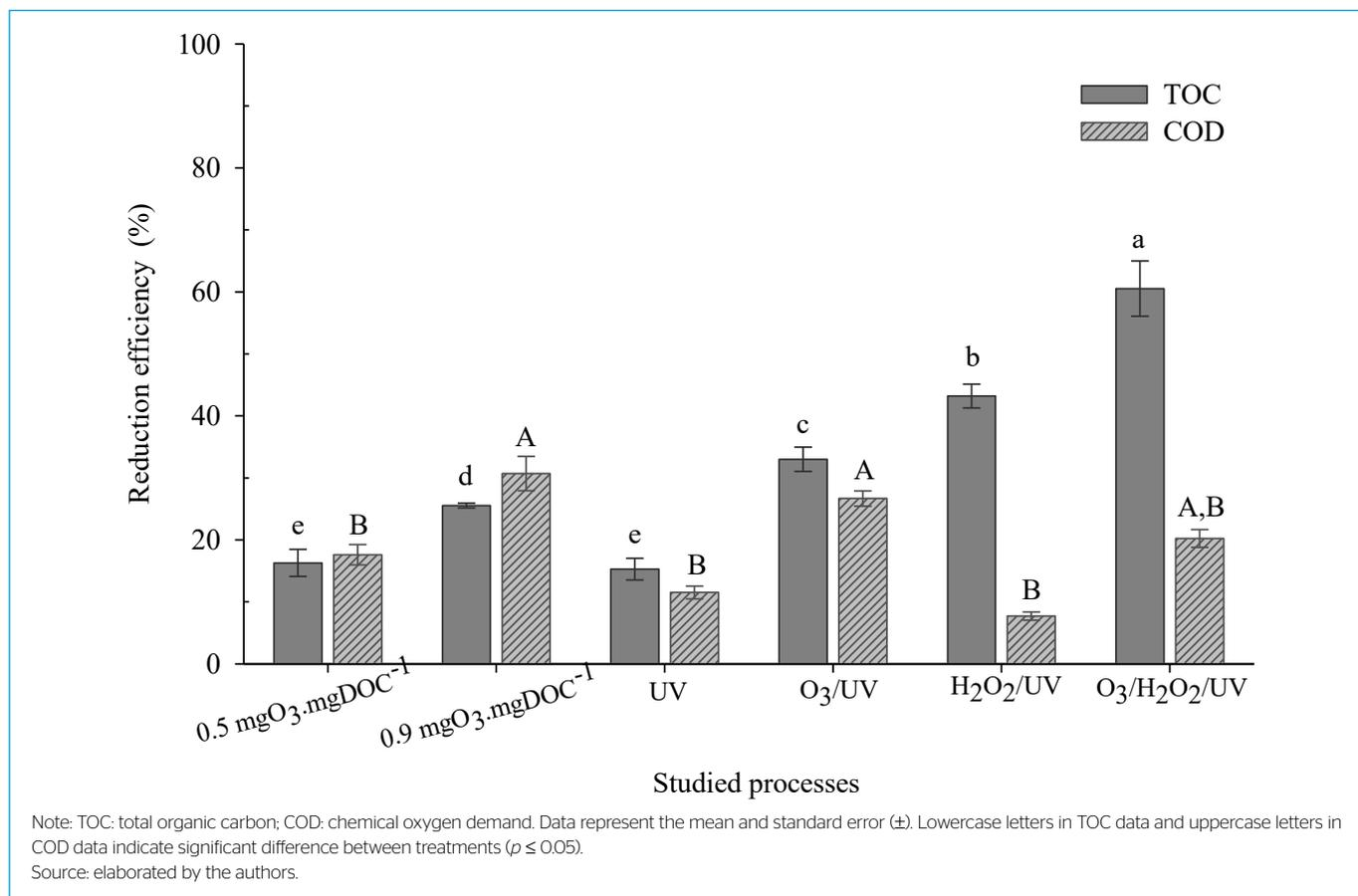
**Figure 4** - Efficiency in reducing total organic carbon and chemical oxygen demand through advanced oxidative processes.
