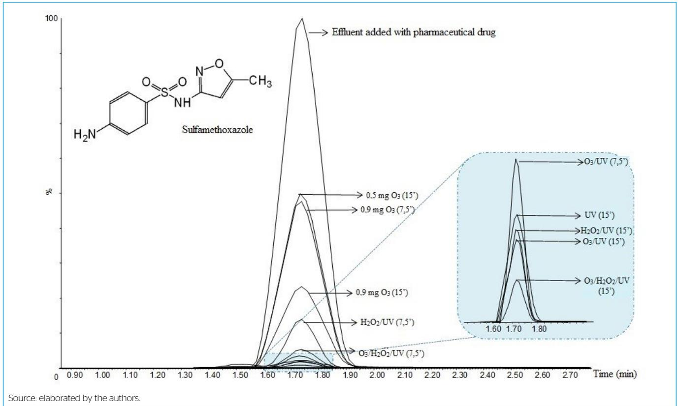
Figure 2 - Total ion chromatogram generated for sulfamethoxazole after effluent treatment based on different advanced oxidation processes.
