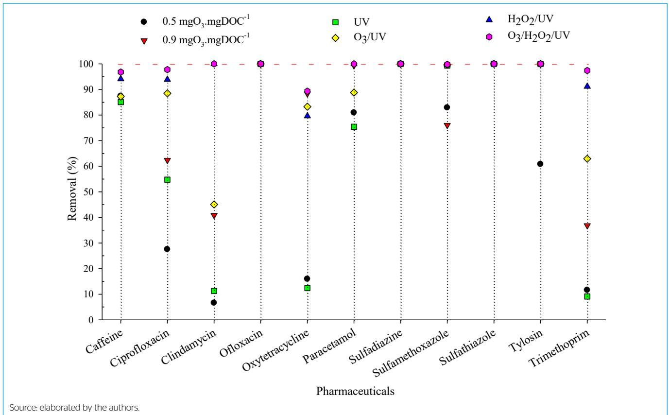
Figure 3 - Removal of the investigated pharmaceuticals through advanced oxidative processes:  $O_3$ /UV (15 W);  $O_3$ /UV (0.5 mg $O_3$ -mgDOC<sup>-1</sup>/UV 15 W);  $H_2O_2$ /UV (25 mg $H_2O_2$ -L<sup>-1</sup>/UV 15 W);  $O_3$ / $H_2O_2$ /UV (0.5 mg $O_3$ -mgDOC<sup>-1</sup>/ 25 mg $H_2O_2$ -L<sup>-1</sup>/UV 15 W)
