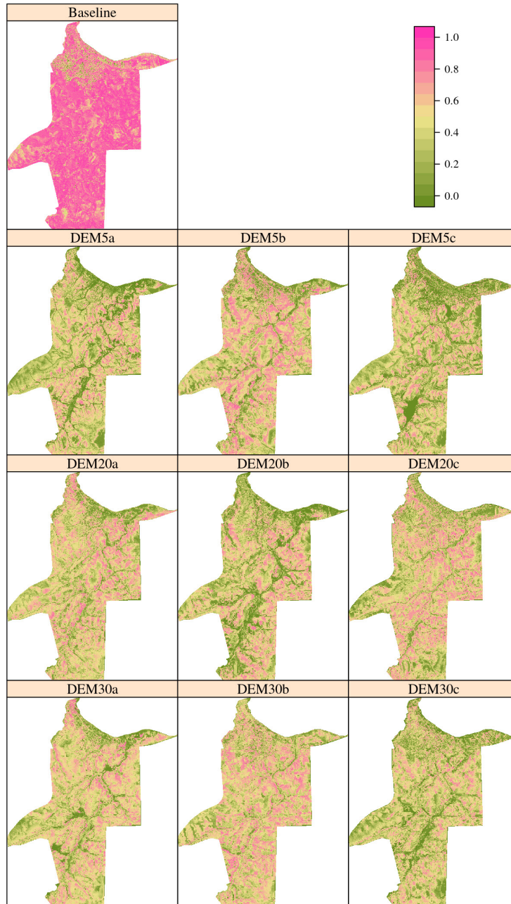
Figure 6: Shannon entropy (uncertainty) of predictions of multinomial logistic regression models calibrated using satellite images (baseline, p = 3 ) and digital elevation models ( p = 13 ) with different levels quality (as defined in this study).
