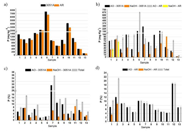
**Figure 2:** P contents of the extracts of the 3051A and aqua regia (AR) (a), P contents of sequential extractions with ammonium oxalate (OA) and NaOH in residues of 3051A and aqua regia (b), and the relative percentages of the contents of these oxides extracted by the sequential extractions with ammonium oxalate and NaOH in relation to the contents extracted from the 3051A (c) and aqua regia (d). Total = content of the P-ammonium oxalate + P-NaOH.
