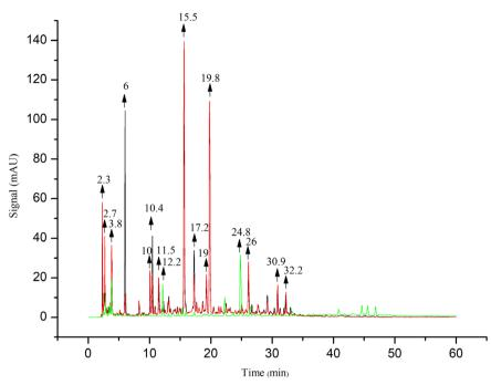
**Figure 1:** HPLC chromatogram of protein extracts from artichoke leaves using the mechanical stirring method. Citrate-MS (black), Acetate-MS (red) and Tris-MS (green).
